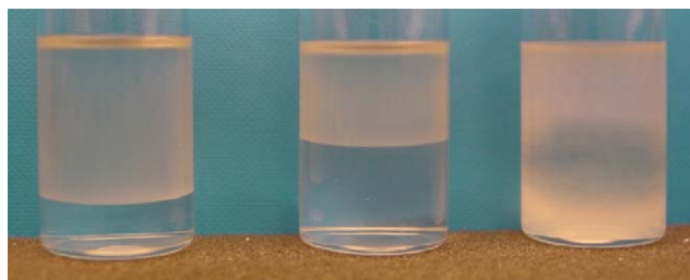
Fig. 7 Mixtures of soy oil (2 ml), water (1 ml) and solvent (4 ml), where the solvent is THF (left), dioxane (centre), or acetone (right).
